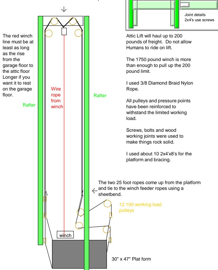
Ropes had a retrace figure8 as a stopper knot and a half hitch used to adjust the height on the bottom of the platform. I just drilled a 3/8" hole and tied a retrace 8 on the bottom..
